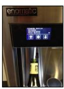
Step 4: Insert the bottle straw inside the new bottle and place bottle on the lifter. Select change bottle (the bottle will raise and seal
