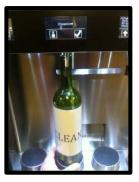
Step 4: Place the cleaning bottle filled up with hot water on the lifter and Press the left icon
