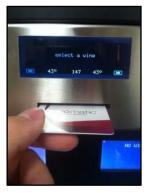
Step 1: The Main Display will read "select wine and a box appear around each glass icon. **Insert the pouring card** in the reader and leave it in place.
