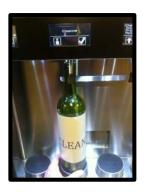
Step 4: Place the cleaning bottle filled up with hot water and citric acid (4 tables spoons or 2 oz ) on the piston and Press the *left icon*
